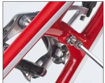
Figure 14. Removing interior screw from brake nut
